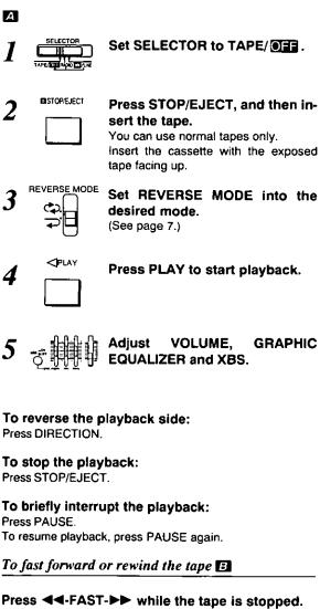
The tape will start moving at high speed. To stop the fast forward or rewind operation, press STOP/ EJECT.
