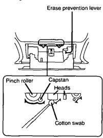
It is recommended that the head assembly be demagnetized if distortion or poor sound quality persists after cleaning the heads.
