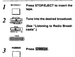
To stop the recording: Press STOP/EJECT.
